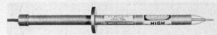
Figure 11. -hp- Model 459A Multiplier permits measurement of voltages up to 30,000 volts d-c.
